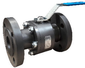
BF Series 2 split body - Floating CI 150 to 600 DN ½" (15) to 6" (150)
