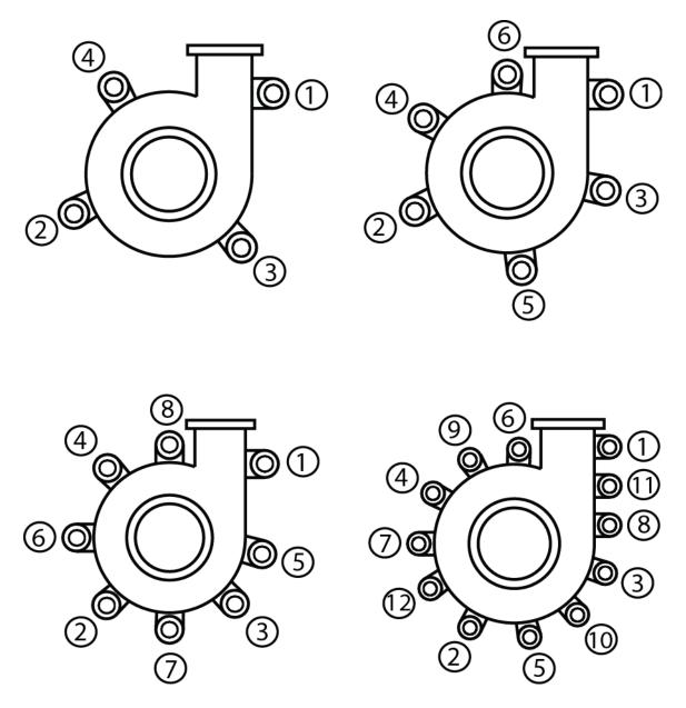
Figure B-1. Cover Plate Bolt Tightening Sequence.
