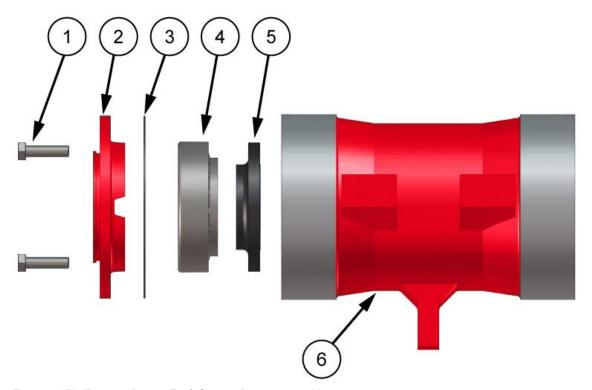
Figure 17. Fitting Drive End Outer Bearing to Housing.
