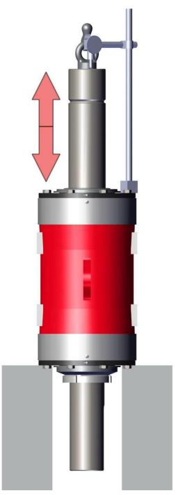
Figure 20. Checking End Play on Heavy Duty Bearing Assemblies.
