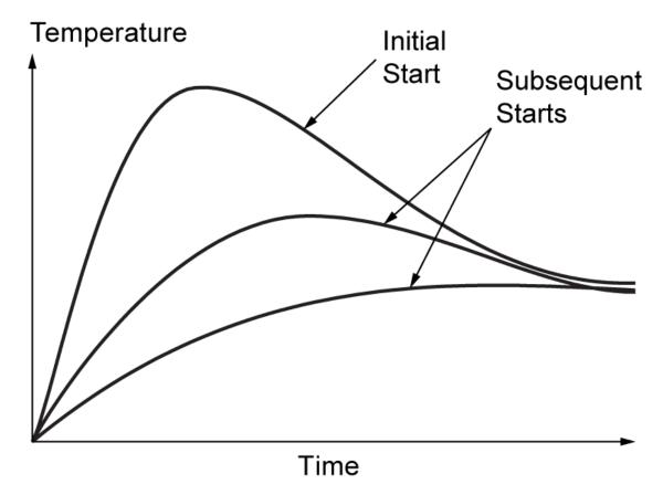
Figure 3. Time versus Temperature Characteristics of a Grease Lubricated Bearing Assembly.
