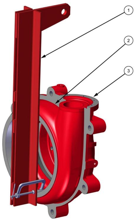
Figure 39. Volute Lifting Beam Installation.
