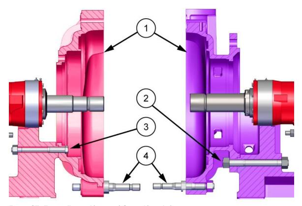
Figure 27. Fitting Frame Plate and Cover Plate Bolts.
