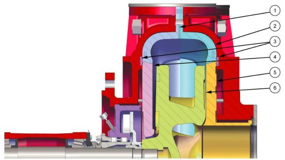
Figure 43. Four Part Separate Rubber. Fitting Frame Plate Liner, Cover Plate Liner, Frame Plate Liner Insert, Throatbush, Volute Liner Seals and Impeller.
