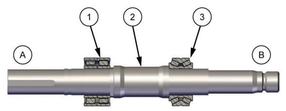
Figure 16. Fitting Drive End and Impeller End Bearing Assemblies.
