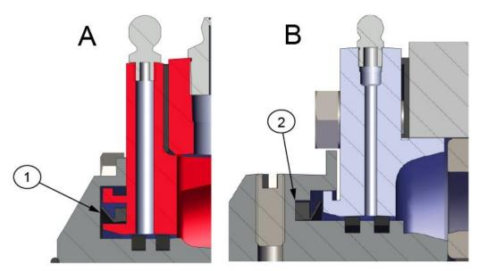
Figure 14. Bearing Seal Rings.
