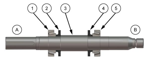
Figure 8. Fitting Grease Retainers and Bearing Cones.
