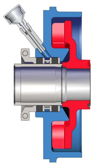
Figure 5. Expeller Ring Arrangement.
