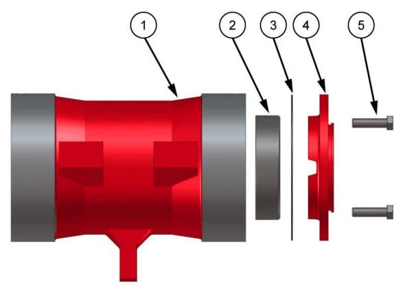
Figure 9. Fitting Wet Bearing Cup to Housing.
