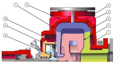
Figure 36. Three Part Metal. Fitting Frame Plate Liner Insert, Volute Liner, Seal Rings, Volute Liner Seals, Impeller O-Ring, Impeller and Cover Plate.
