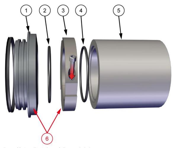
Figure 22. Impeller Release Collar, exploded view.
