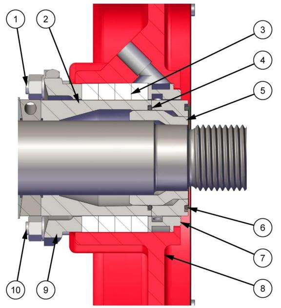
Figure 29. Gland Seal Cross Sectional View.
