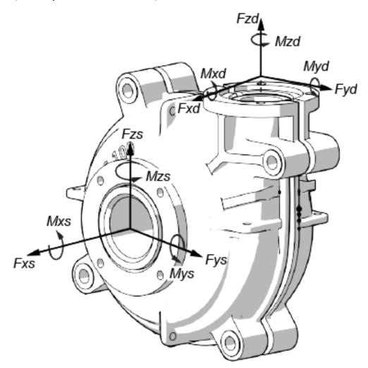
Figure D-1. Direction of forces and moments being applied to suction and discharge nozzles.
