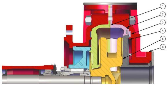
Figure 42. Three Part Separate Rubber. Fitting Frame Plate Liner, Cover Plate Liner, Throatbush, Volute Liner Seal, Impeller and Cover Plate.
