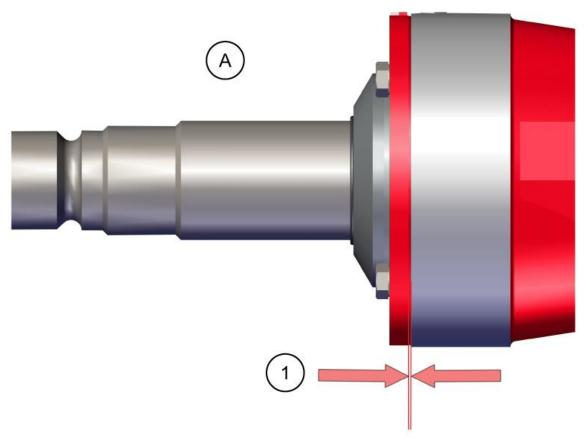
Figure 10. Gap Measurement.
