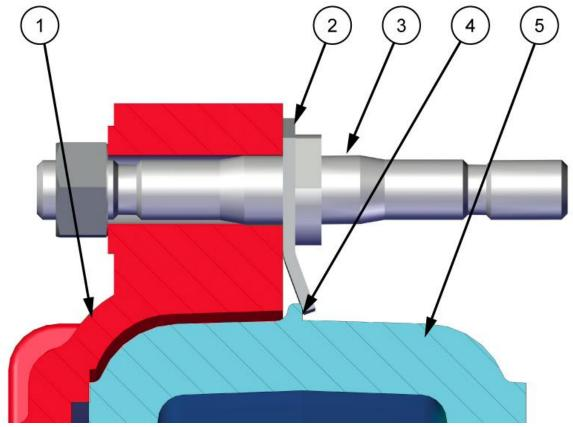
Figure 37. Using Keeper Plate to Retain Volute.
