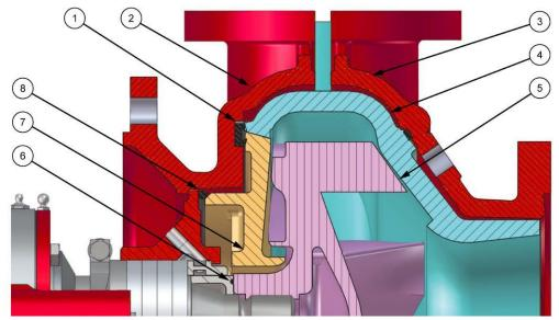
Figure 35. Two Part Metal. Fitting Seal Ring, Frame Plate Liner Insert, Volute Liner Seals, Impeller, Volute Liner and Cover Plate.
