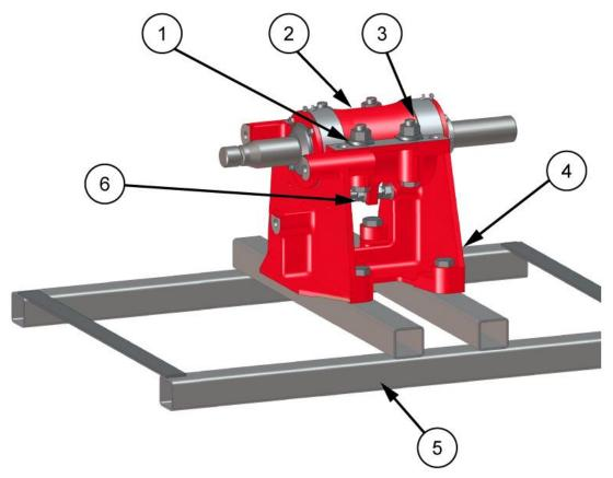
Figure 25. Fitting Bearing Assembly to Base.
