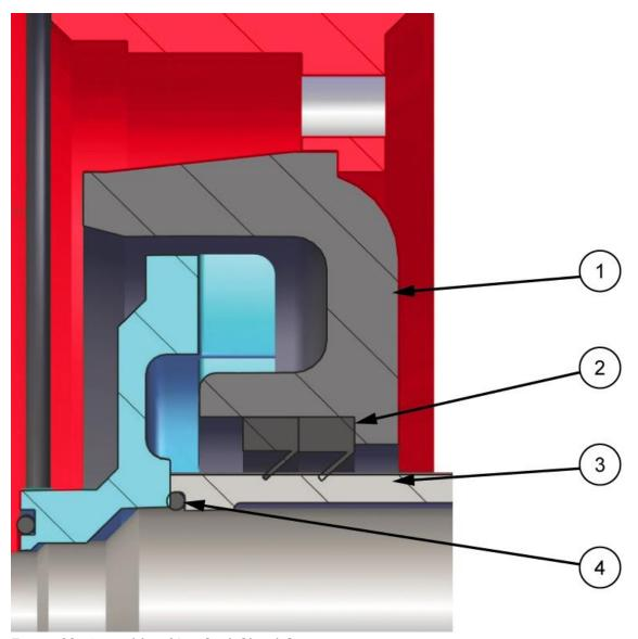
Figure 32. Assembly of Lip Seal Gland Components.
