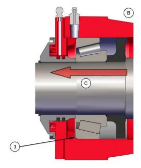
Figure 11. Adjustment of Bearing Cup.
