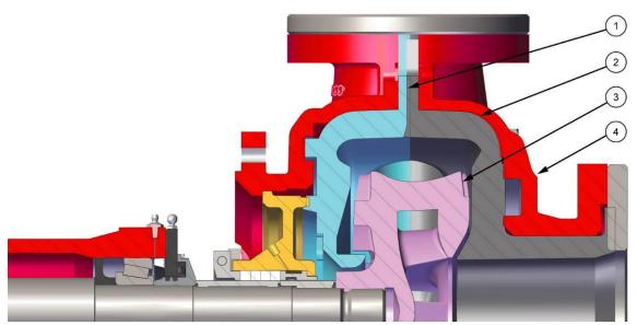
Figure 40. Two Part Rubber. Fitting Frame Plate Liner, Cover Plate Liner, Impeller and Cover Plate.
