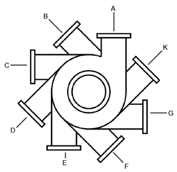
Figure 26. Discharge Orientation as Established by Frame Plate Assembly, facing suction side.
