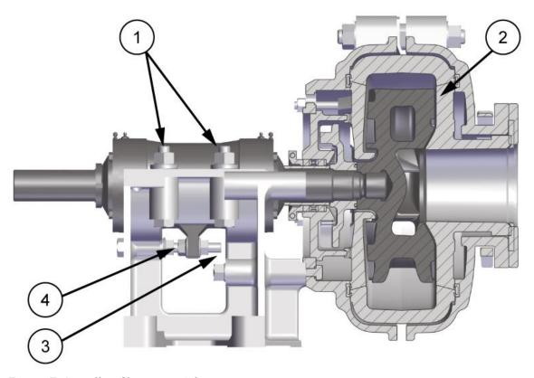
Figure 7. Impeller Clearance Adjustment.
