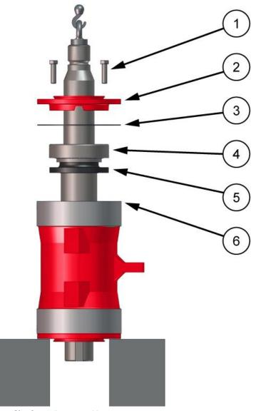
Figure 18. Fitting Shaft to Bearing Housing.
