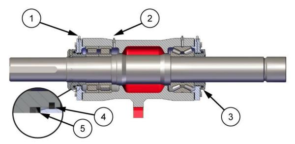
Figure 19. Fitting Labyrinths, V-Rings, Piston Rings on Heavy Duty Bearing Assemblies.
