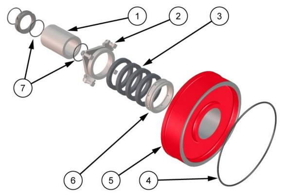
Figure 28. Gland Seal Assembly Exploded View.
