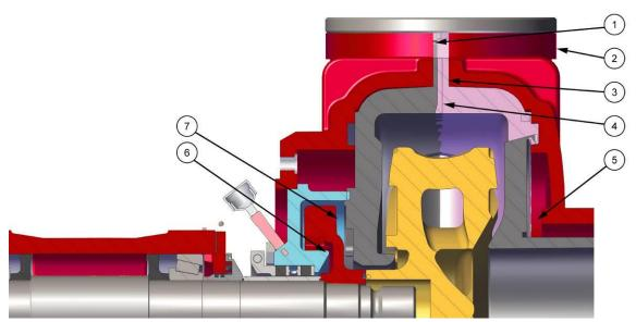
Figure 41. Three Part Integral Rubber. Fitting Frame Plate Liner, Cover Plate Liner, Throatbush, Impeller and Cover Plate.
