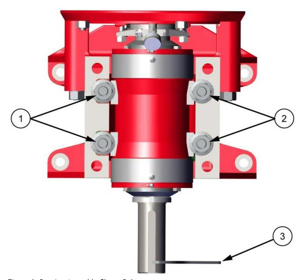
Figure 6. Bearing Assembly Clamp Bolts.
