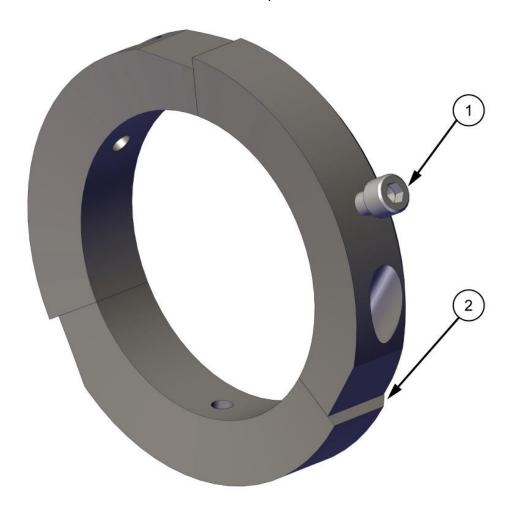
Figure 24. Segmented Release Collar.
