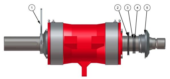
Figure 15. Fitting Labyrinths, Piston Rings and Locknuts
