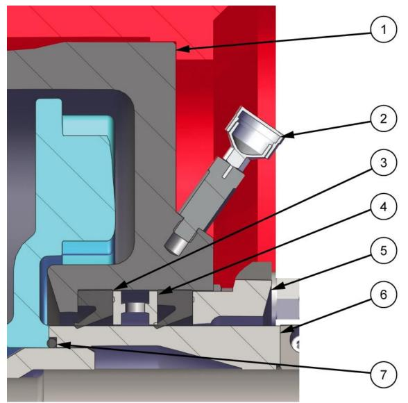
Figure 34. Fitting of Expeller Ring, Shaft Seals, Gland Studs, Gland, Shaft Sleeve, Shaft Sleeve O-Ring and Expeller.
