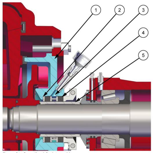
Figure 31. Centrifugal Seal Assembly.
