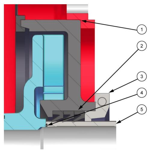
Figure 33. Fitting of Expeller Ring, Shaft Seals, Gland Studs, Gland, Shaft Sleeve, Shaft Sleeve O-Ring and Expeller.
